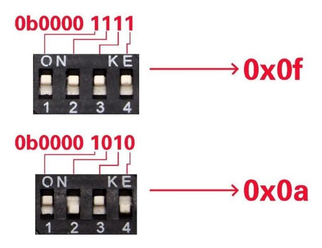
Then keep the address setup in the program the same as the address setup on the I2C motor driver. The default address setup in the program is 0x0f.
