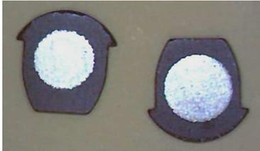
CONDENSATEUR CHIP TYPE DISQUE 15pf.
