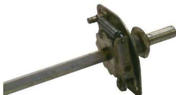
MECANISME COMMUTATEUR ROTATIF AVEC SABRE.
