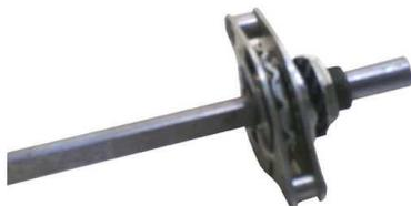
MECANISME COMMUTATEUR ROTATIF AVEC SABRE.
