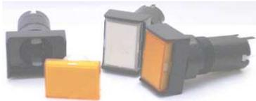
VOYANT RECTANGULAIRE ORANGE/BLANC (CABOCHONS INTERCHANGEABLES) POUR LAMPE MIDGET GROOVED. AVEC POUSSOIR ON/ON, 1 INVERSEUR. PERCAGE 16mm. DIM.: 24x18x46mm.
