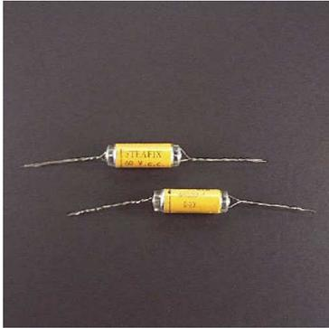
CONDENSATEUR STYROFLEX DOUBLE.
